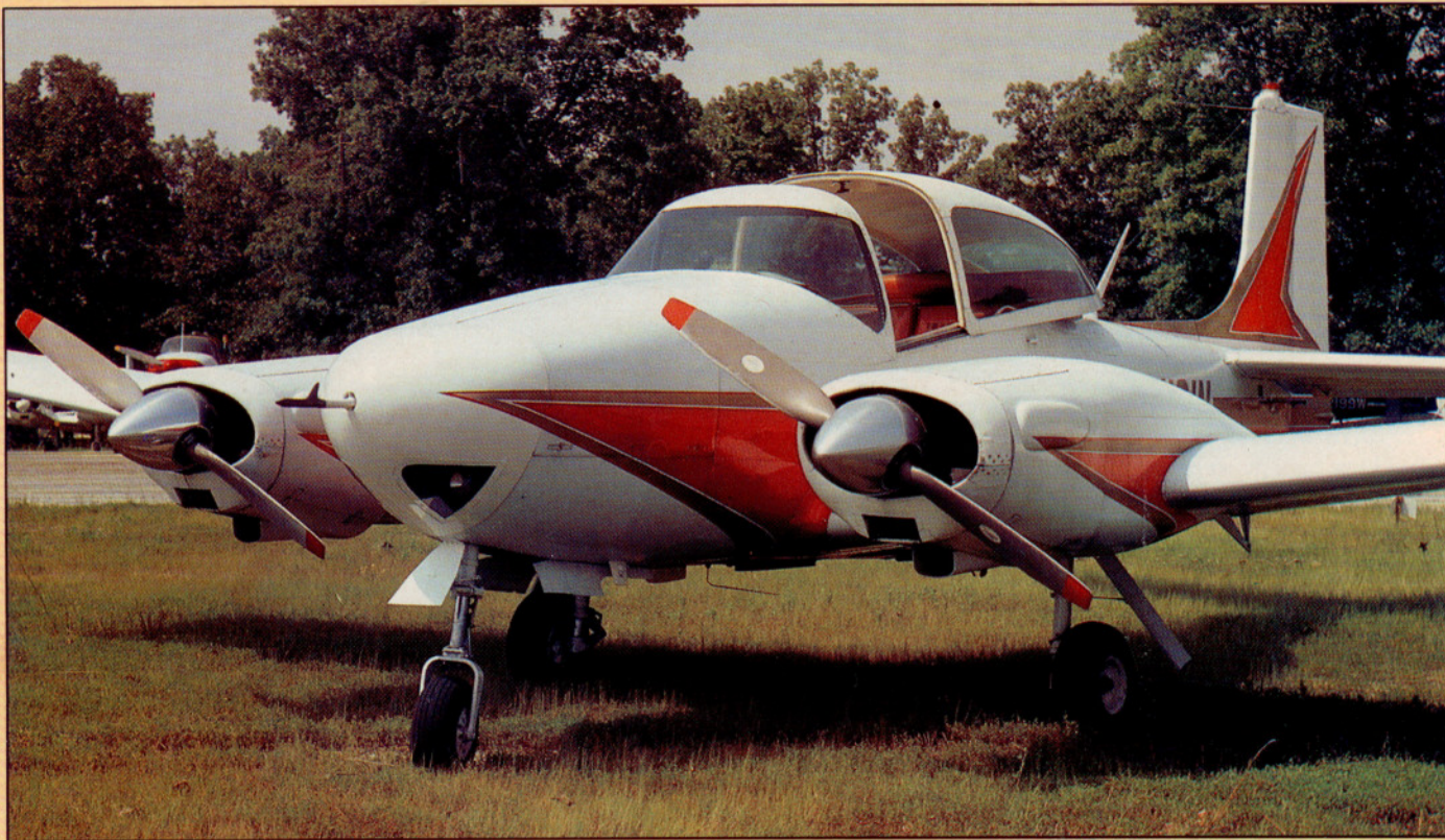
Riley Aircraft certificated the first Navion twins, with 150/160-hp Lycomings. Temco and Cameron Iron Works also do twin conversions now. About 125 are flying.
